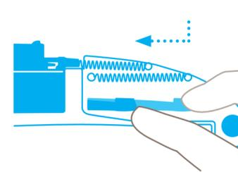
Release the blade carrier by **pressing down and pushing forward**, as indicated.
