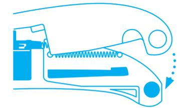
Finally, fold the **upper half of the handle back down** until it snaps into place. Please check blade retraction!
