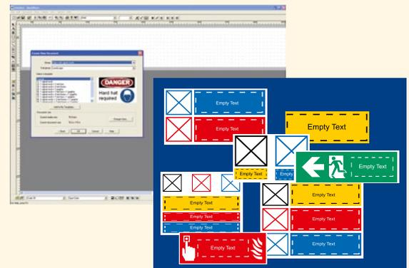
Includes label template designs. The size of the template adjusts automatically to the size of the installed adhesive roll, regardless of width.
