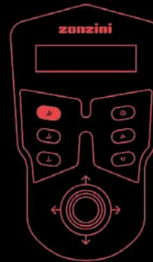
Top left button of the joystick. The crawler tracks close completely and allow the wheels to rest on the ground, it helps to turn on narrow stairs and kite winder steps.
