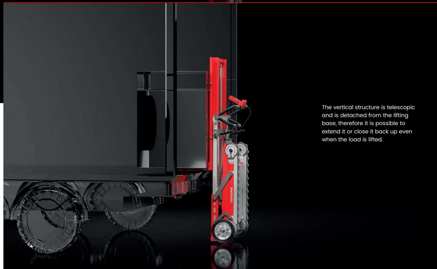
The vertical structure is telescopic and is detached from the lifting base, therefore it is possible to extend it or close it back up even when the load is lifted.
