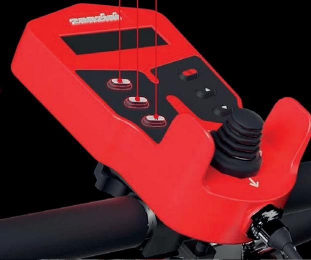
Crawler tracks in maximum opening position. Third button on the bottom left of the joystick.
